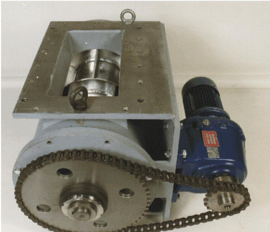
These compact locks are robust welded constructions with **continuously variable inlet and outlet dimensions** - from 150 x 150 mm to 400 x 800 mm - and **discharge rates of 1,7 to over 200 m<sup>3</sup>/h (at 100 % fill)**. They are ideal for discharging large quantities of bulk materials from silos, bunkers and other equipment.
