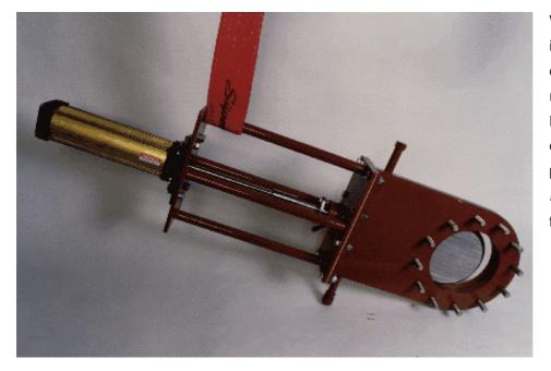
Water-cooled slide gates as intermediate-flange-type in welded construction made of temperatureresistant steels, heat-resistant steels or Ni-based alloys, designed for tube diameters *DN 100 - DN 500* with the purpose of *shutting off hot bulk materials up to 1000* ° *G* by variable flange sizes also usable in lined pipings.
