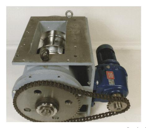
These compact locks are robust welded constructions with **continuously variable inlet and outlet dimensions** - from 150 x 150 mm to 400 x 800 mm - and **discharge rates of 1,7 to over 200 m3/h (at 100 % fill)**. They are ideal for discharging large quantities of bulk materials from silos, bunkers and other equipment.
